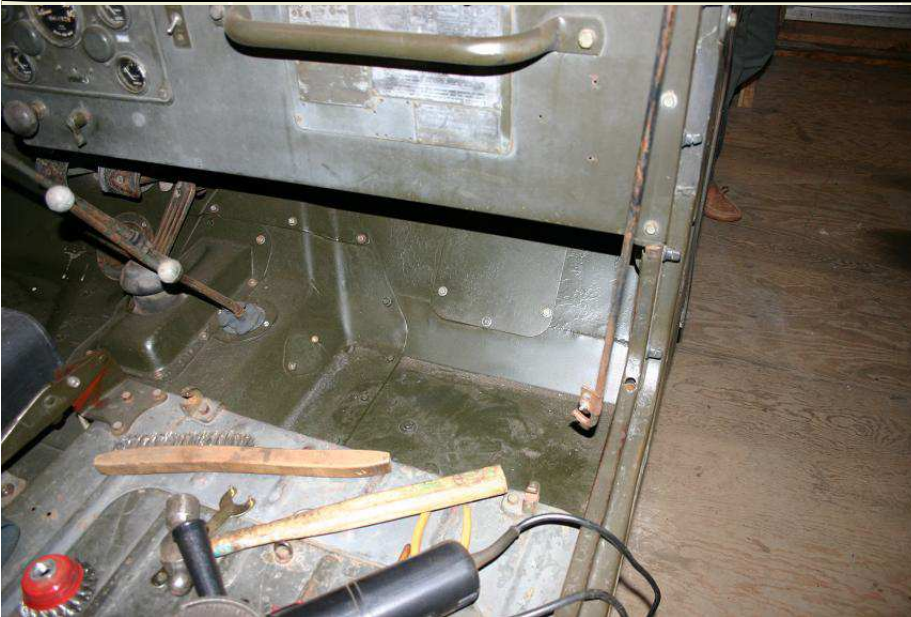
New M38 Floor Installed in Don's Jeep
