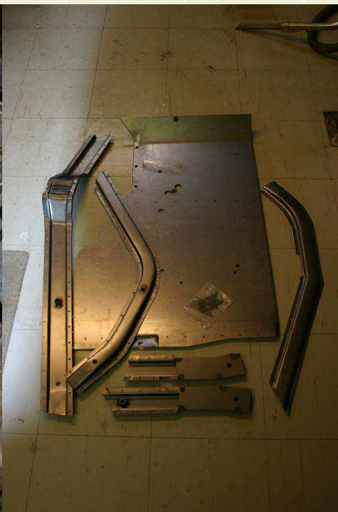
Don Trueman's M38A1 gets prepped for a "floorectomy" with the replacement parts from Midwest Military ready to go in.
