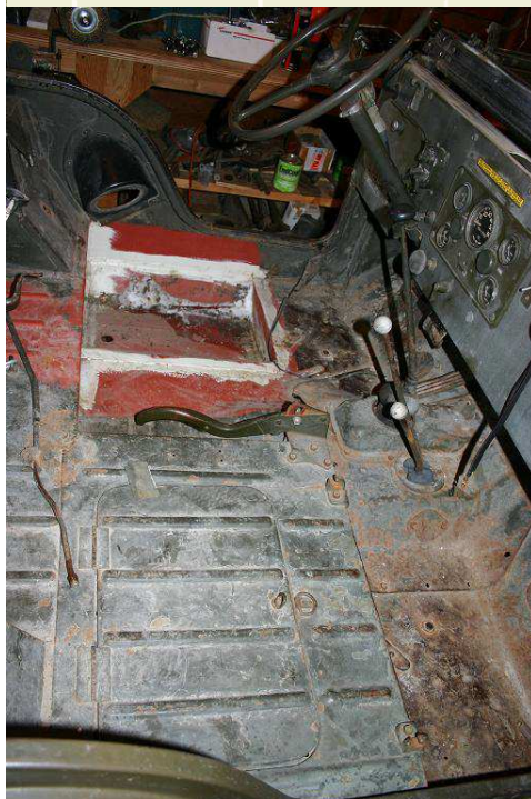
Don Trueman's M38A1 gets prepped for a "floorectomy" with the replacement parts from Midwest Military ready to go in.
