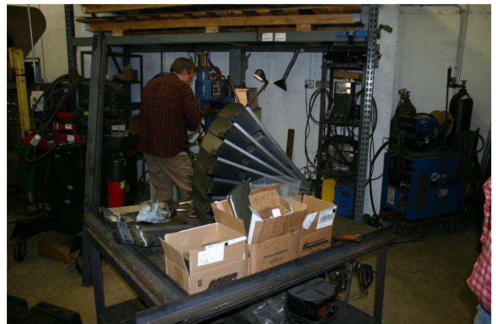
Midwest employee Al Lehmann spot welds another M38A1 fuel tank well - one of Midwest's products
