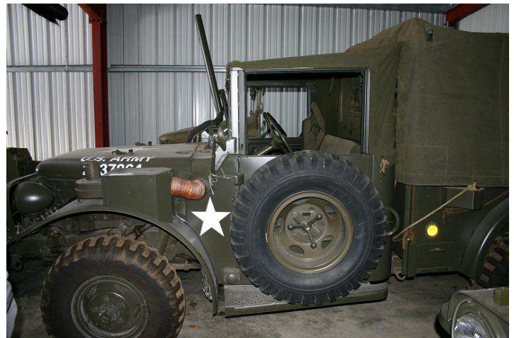
John's M42 Command vehicle with modified breather pipe.
