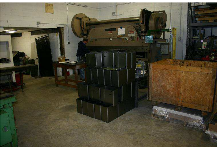
Midwest employee Karl Holm at the brake press adding to the rapidly growing stack of M38 cowl battery boxes.
